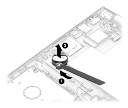
Reverse this procedure to install the RTC battery. When installing the RTC battery, make sure the "+" sign is facing up.
