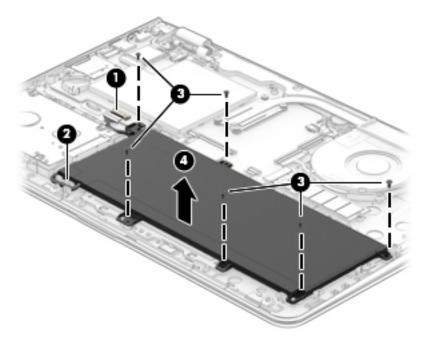
Reverse this procedure to install the battery.
