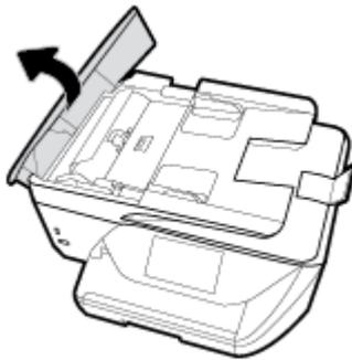
2. Lift the tab located on the front edge of the document feeder.
