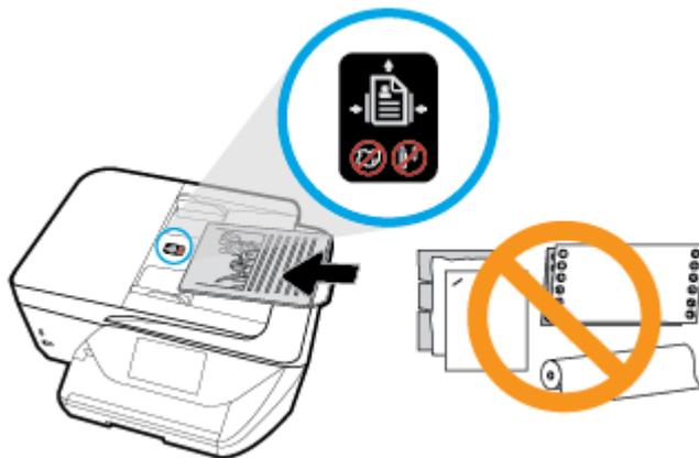
3. Slide the paper-width guides inward until they stop at the left and right edges of the paper.
