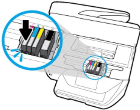
Make sure that the color-coded letter on the cartridge matches that on the slot.
