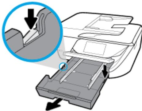
4. Check the gap in the printer where the input tray was. If there is any jammed paper, reach into the gap, grasp the paper with both hands and pull it towards you.
