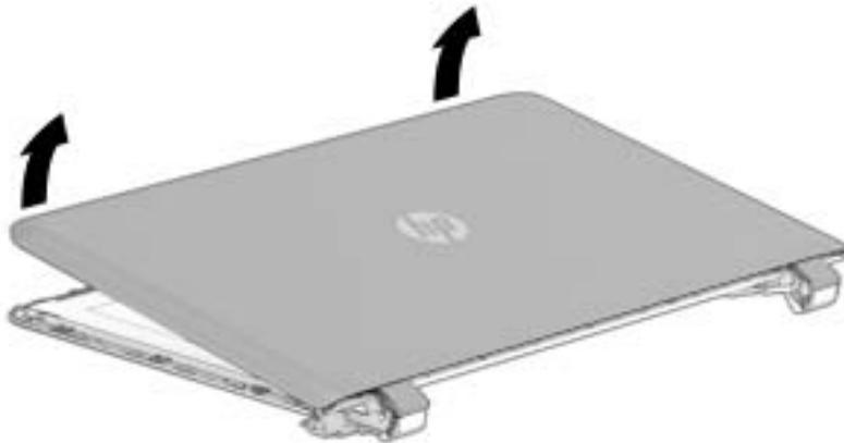
2. Turn the display with the bezel down and the back of the panel up. Disconnect the display cables from the panel and bezel **(1)**, **(2)**. Release the connections **(3)**, **(4)** and lift the panel **(5)**.
