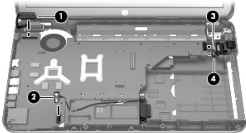
2. Remove the PM 2.5 × 4.5 screw (1) that secures the system board to the base enclosure.
