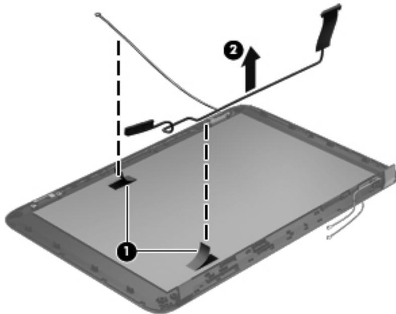
10. If it is necessary to replace the wireless antenna cables and transceivers:
