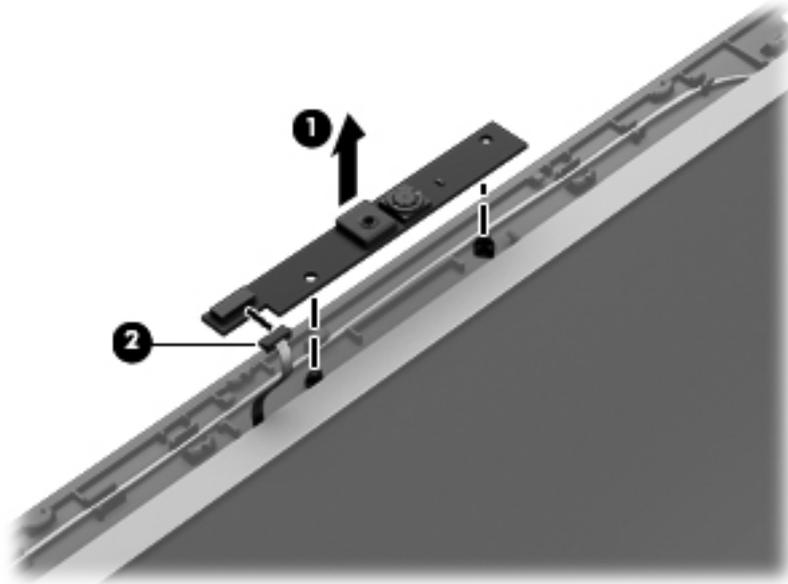
7. If it is necessary to replace the display panel:
