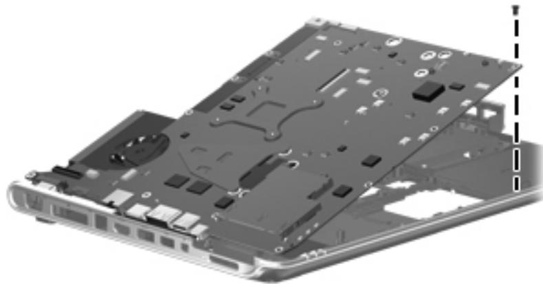
**Where used:** One screw that secures the system board to the base enclosure
