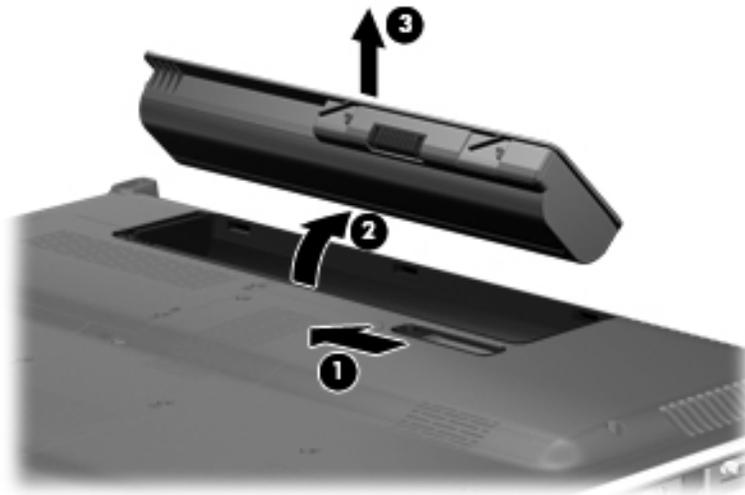
To install the battery, insert the rear edge of the battery into the battery bay and pivot the front edge of the battery downward until it is seated. The battery release latch automatically locks the battery into place.
