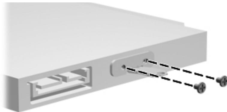
**Where used:** 2 screws that secure the mounting bracket to the hard drive
