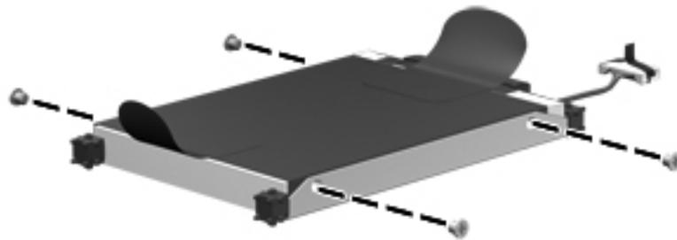
**Where used:** 4 screws that secure the hard drive brackets to the rail
