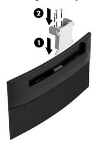
3. Secure the mounting plate to the wall or swing arm of your choice using the four screws included with the VESA mounting bracket.
