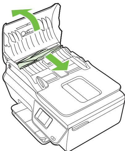
2. Lift the tab located on the front edge of the ADF.
