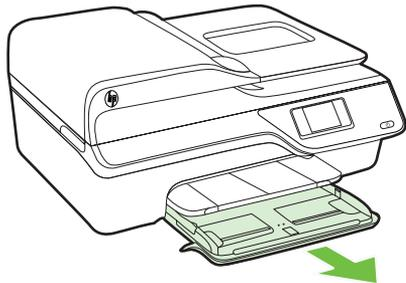
2. Slide out the paper width guides in the input tray as far as possible.
