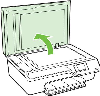
3. Clean the glass and lid backing by using a soft, lint-free cloth that has been sprayed with a mild glass cleaner.
