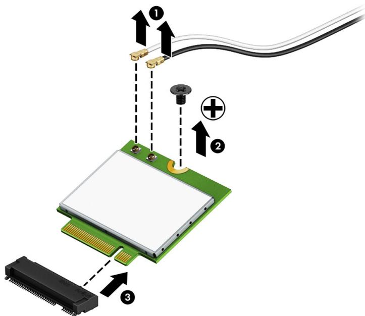
Reverse this procedure to install the WLAN module.
