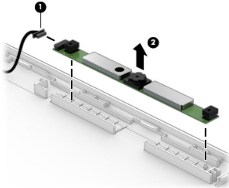
Reverse this procedure to install the webcam.
