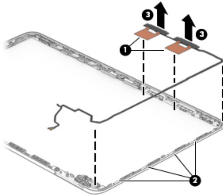
Reverse this procedure to install the WLAN antenna cable.
