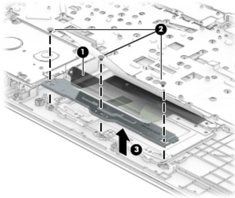
3. Disconnect the TouchPad cable, and then remove the metal shield covering the TouchPad (1).
