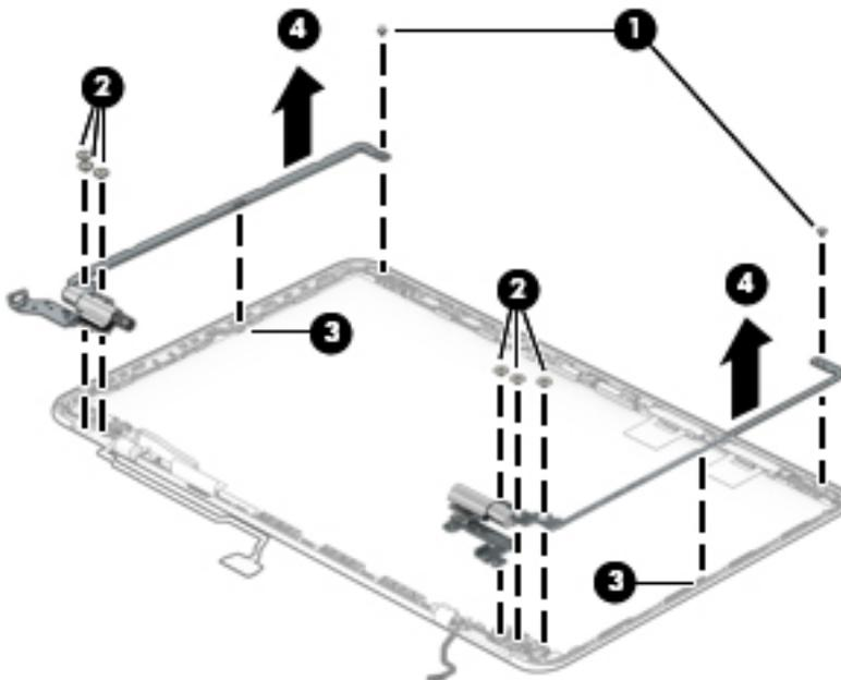
4. Remove 1 Phillips 2.0x2.0 screw from each hinge cover (1) separate the hinge covers (2) from the back cover (3), and then lift the hinge covers (4) to remove them.
