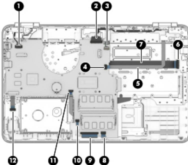
2. Remove 2 Phillips 2x5 screws (1), and then lift the system board to remove it (2).
