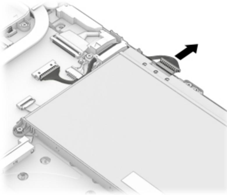
2. Remove 3 Phillips 2x5 screws (1), and then lift the battery to remove it (2).
