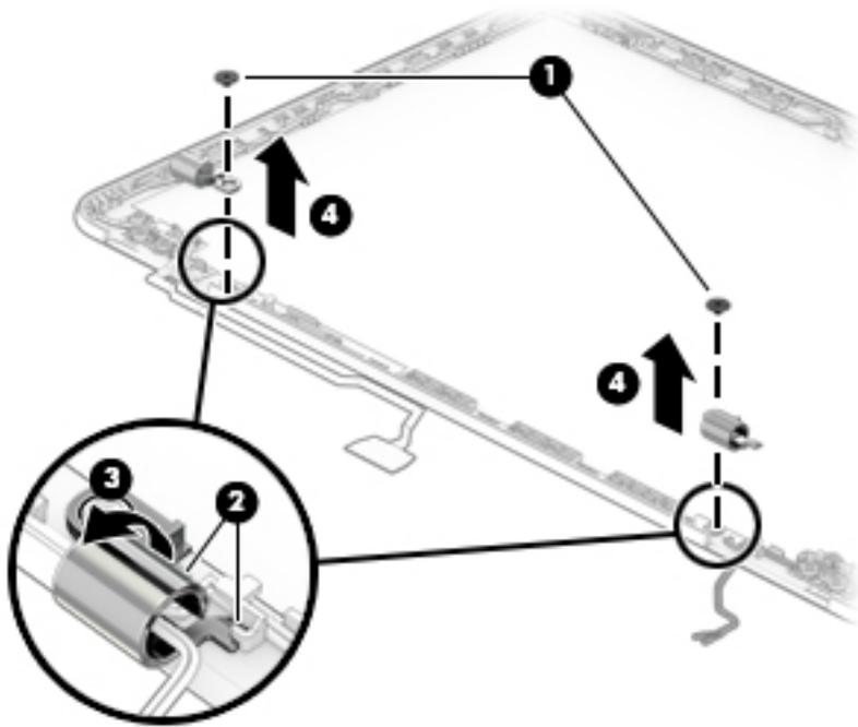
5. Remove 4 Phillips 2.0x2.5 screws from the display panel (1), and then lift the display panel (2) to remove it.
