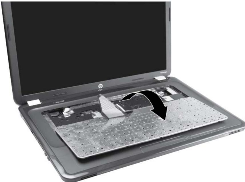
4. Release the zero insertion force (ZIF) connector **(1)** to which the keyboard cable is attached, and then disconnect the keyboard cable **(2)**. Remove the keyboard **(3)**.
