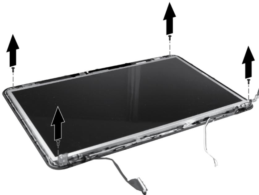
15. Tilt the display **(1)** up, release the tape **(2)** holding the display cable to the display panel, and then disconnect the cable **(3)**.
