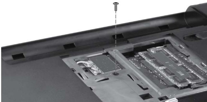
2. Open the display and stand the computer on its side. Insert a small screwdriver through the keyboard access hole in the bottom of the computer. (The keyboard access hole is the same hole from which the keyboard screw was removed.) Push firmly on the bottom of the keyboard until it is disengaged.
