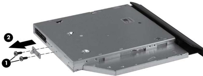
7. To replace the optical drive bezel, disconnect it from the optical drive.
