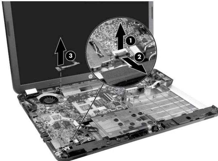
Reverse this procedure to install the TouchPad LED board.
