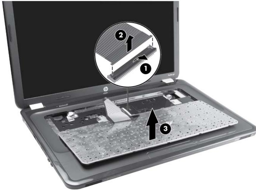
Reverse this procedure to install the keyboard.
