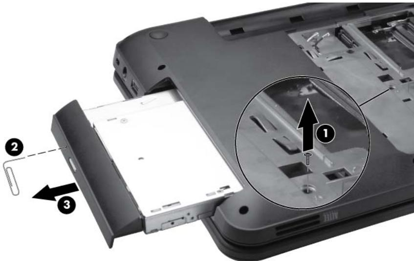
4. To replace the optical drive bracket, position the optical drive with the optical drive bracket toward you.
